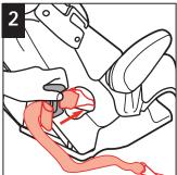
LATCH adjuster can be on either side, but belt should not be twisted.
